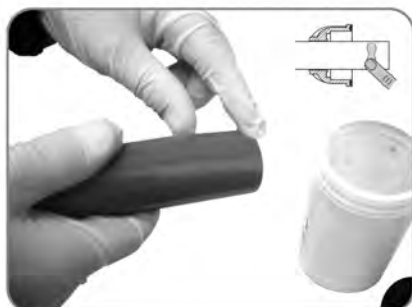
Lubricate the outer part of the pipe
